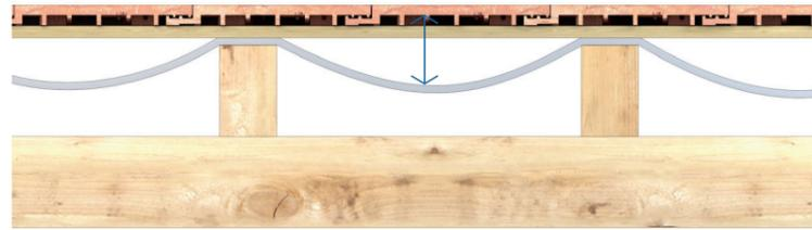
b) When laid fully supported over rigid sarking or insulation, install 50 x 25mm counter battens, fixed directly into and over the rafters or trusses to provide a drainage path and batten cavity ventilation. Install nail tape between each counter batten and underlay.
